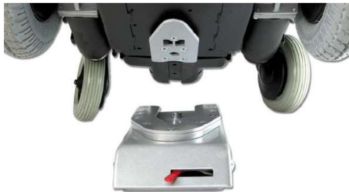
Docking station and docking plate on chassis
