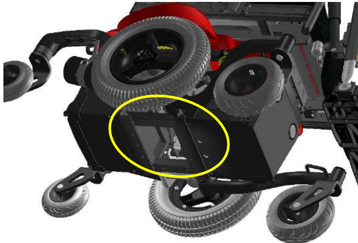
dedicated holes for mounting Dahl mounting plate
