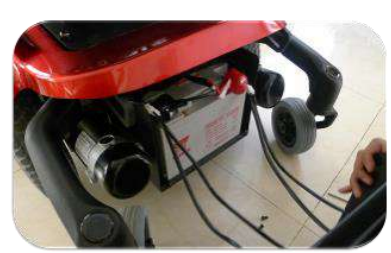
position of the rear battery (behind both covers)
