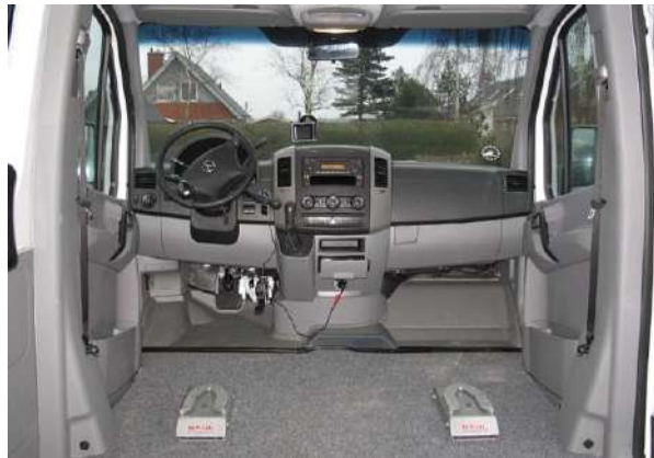
Dahl docking station mounted on the floor
