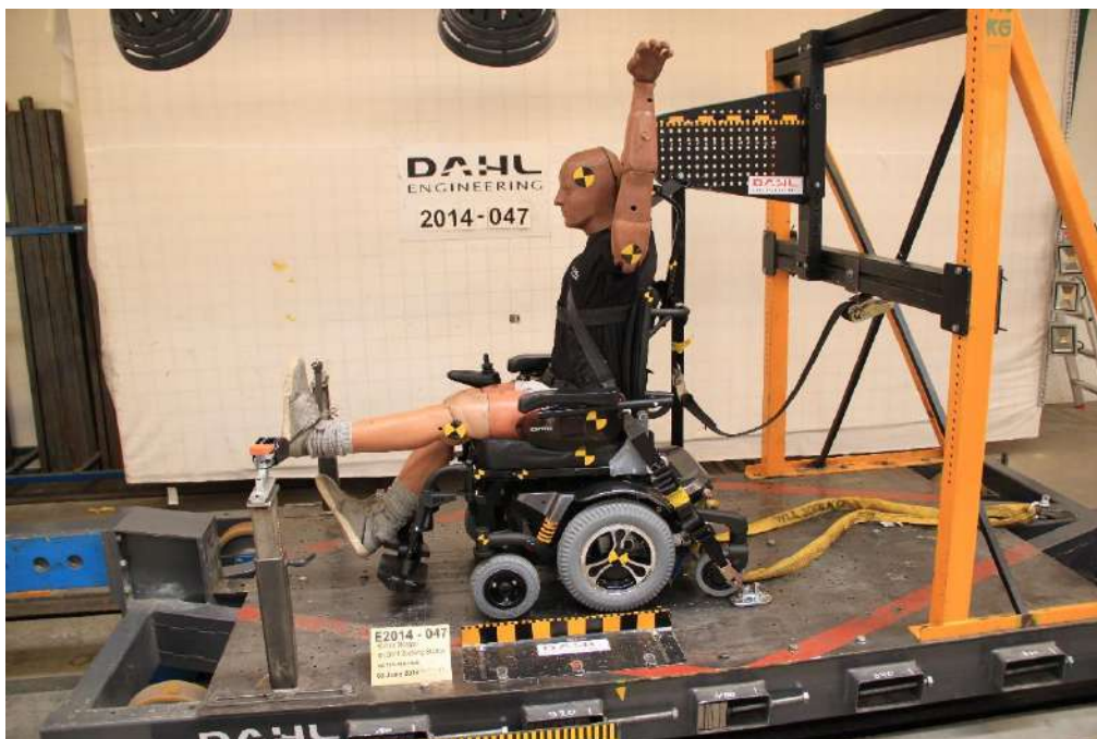
Morgan crash test using Dahl Docking station.
